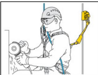
Allows the rope to be kept at a distance to protect it during certain work phases.
