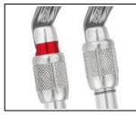
To facilitate equipment checks, SCREW-LOCK manual locking carabiners have a red band that is visible only when the carabiner is not locked.
