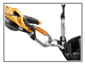
The Am'D carabiner has an asymmetric D shape that is ideal for attaching equipment such as descenders or positioning lanyards. Usage of the CAPTIV positioning bar favors loading of the carabiner along its major axis, limits flipping and keeps it attached to the device or lanyard.
